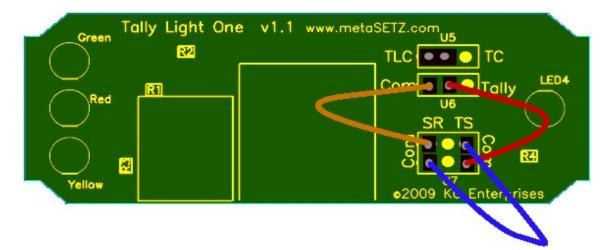
In this mode the four LEDs can be independently controlled by the TLC-6 and the 3.5mm jack can be used as an intercom or headphone feed for the camera operator. (See TLC-6 manual for details). Connect the TL-1 using the RJ-45 jack and standard Ethernet style cable.
