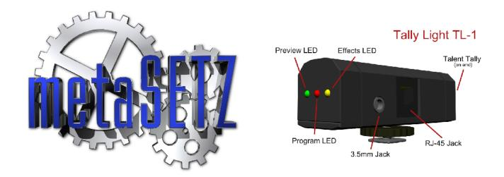
Used in conjunction with the TLC-6 Tally Light Controller and any SD NewTek TriCaster<sup>™</sup> or VT[5]<sup>™</sup> the TL-1 will illuminate LEDs to indicate on which switcher buses an input is active. This is used to inform the camera operator of his cameras status on the switcher. The bright 'Talent' tally can be used to tell the on-camera talent when a particular camera is live.
