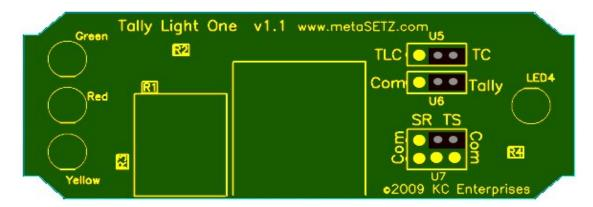
In this mode only the Red 'Program' and 'Talent' tallys will illuminate. If you wish to disable the 'Talent' tally remove the jumper from U5. Connect the TL-1 to the TLC-3 using mono 3.5mm plugs. The TLC-3 uses the tip and sleeve of the mono plug.
