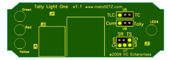
In this mode only the Red 'Program' and 'Talent' tallys will illuminate. If you wish to disable the 'Talent' tally remove the jumper from U5. Connect the TL-1 to the TriCaster using stereo 3.5mm plugs. The TriCaster uses the sleeve and ring of the stereo plug.
